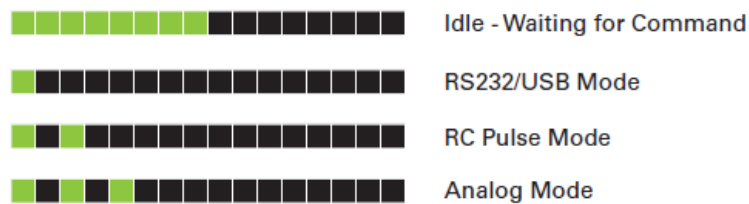
FIGURE 11. Normal Operation Flashing Patterns
